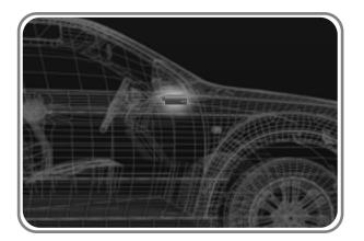
If possible mount the Drone in such a way that the LED's are visible for future troubleshooting. Observe caution when mounting to avoid tension on the harness as it may come loose or damage the unit and/or harness.
