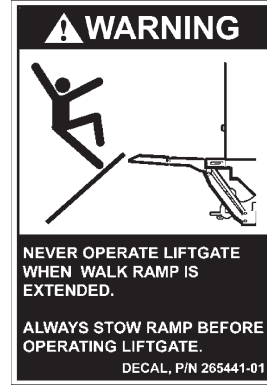
WALK RAMP WARNING DECAL P/N 265441-01
