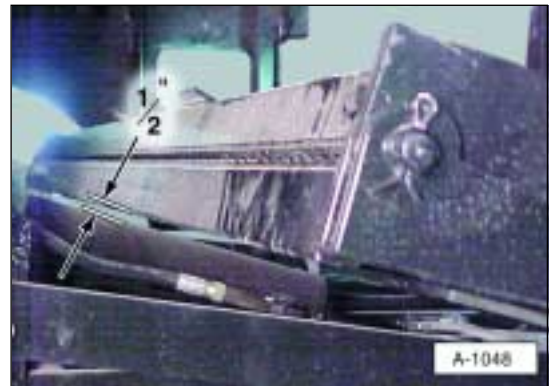
Illustration 17a. Adjust liftgate until there is a 1/2" gap between the cylinder and the liftgate.
