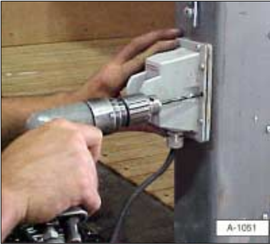
Illustration 19. Install the control switch.
