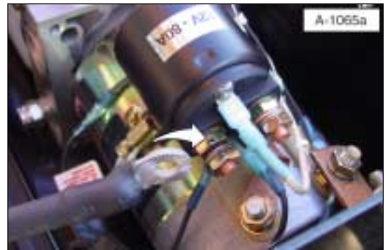
Illustration 8c. Connect power cable to motor solenoid.
