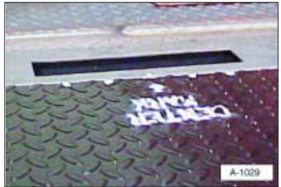
Illustration 4a. Align floor extension with mark.
