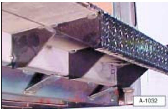
Illustration 4c. Tack weld floor extension brackets.
