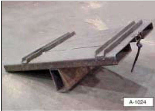
Sample lifting jig.
