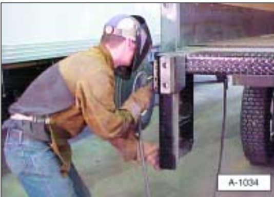
Illustration 20b. Tack weld dock bumpers.
